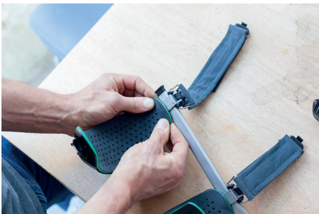
5. Remove the yellow cover to stick the foam to the surface and press tightly.
