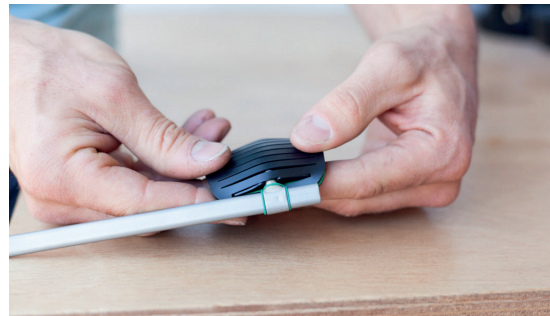
4. Push the flaps properly through the groove so they are visible on the outside.
