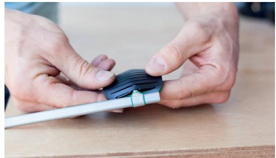
4. Push the flaps properly through the groove in order to make them snap in place so they are visible on the outside.
