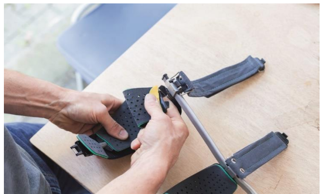
4. Shape to an S-bend. Press the flaps of the inner shell through the outer groove of the outer shell.
