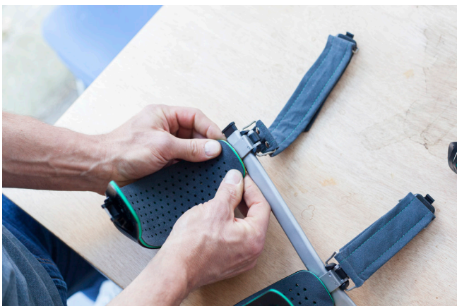
5. Remove the other yellow strip so that the adhesive strip is exposed. Press the adhesive strip well.
